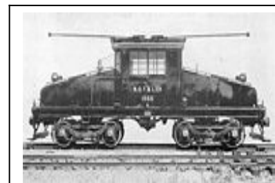
A GE steeplecab electric locomotive. This example is fitted with trolley poles for service on an interurban railroad.
