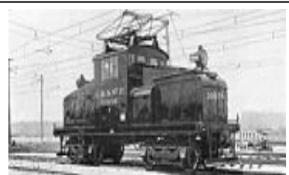
A Milwaukee Road class ES-2, an example of a larger steeplecab switcher for service on an electrified heavy-duty railroad
