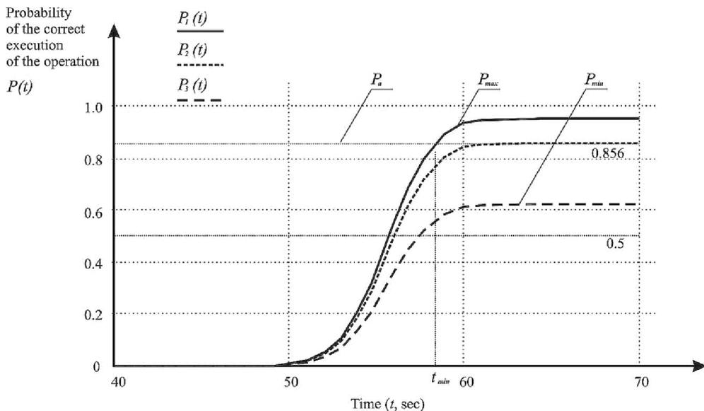
Fig. 4. Execution probability of switching the point from the time of t execution when the psychophysiological condition is changing.
