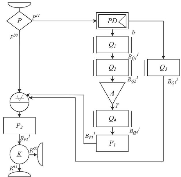
Fig. 1. Functional-semantic network of the performance of the DSP operation when moving the point with false clear of the track area.
