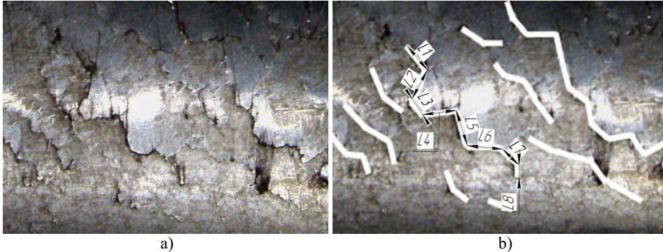
Fig. 1. Determination of the size of contact fatigue defects by analyzing pictures taken by a digital microscope: a) – the picture to be analyzed; b) – the analysis of the picture regarding the average size of the contact fatigue defects; L_1-L_n – the lengths of the defects
