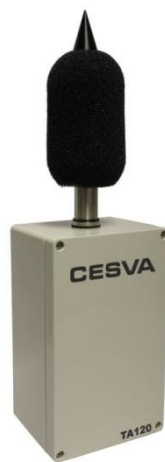
Pic. 1 The TA120 noise measuring sensor for Smart Solutions. Sensor combine the precision of a Class 1 sound level meter, maximum protection of an outdoor kit and full connectivity with CESVA Noise Platform and open source platforms [2]
